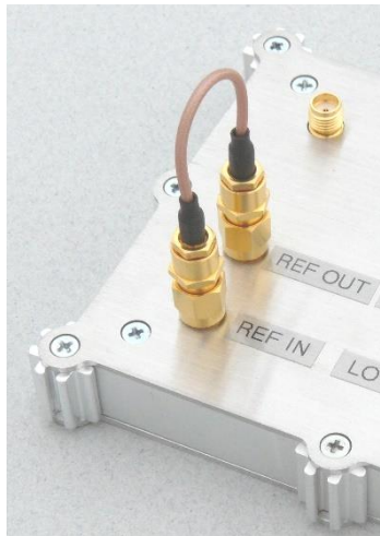
Picture 3-5: Installing the frequency reference SMA interconnect cable for internal frequency operation
