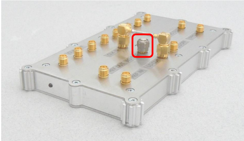
Picture 2-9: SMA terminator (marked in red) factory pre-installed on the secondary sampling clock oscillator output
